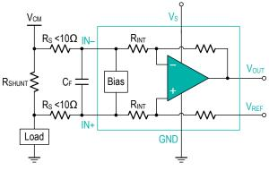
Figure 2. Filter at Input Pins
